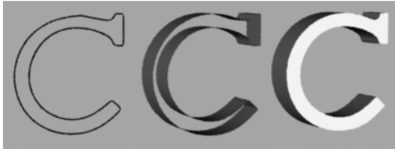
Figure 57: Extrude Object (left: Curve, middle: normal Extrusion, right: Extrusion with Caps)
