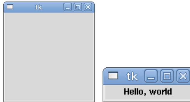
Figure 2.3: Outputs of (a)tkmain.py (b)tklabel.py
